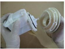
Step1:Disassemble Jet: Pull off "pin lock" Twist motor pump "clockwise" to detach housing and pump. Remove the lock Nut
