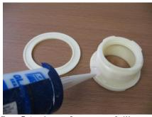
Step 5 Apply good amount of silicon on plastic housing as picture shown above
