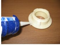
Step 7: Apply second layer of silicon on top of the ring as picture shown Use finger to smooth silicon as needed
