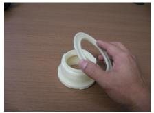
**Step 6**: Place the adapter ring onto housing and top of silicon. Wipe out any residue of silicon before it dries out.
