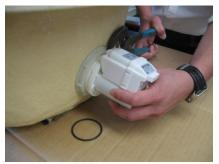
Step 11 Holding housing: Remove the rubber Step 12. Remember to return Black gasket gasket from motor pump. Lock pump to housing "counter-clockwise". hold pump tight while tightening the lock nut
