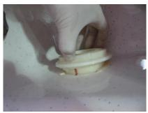
Step8: Install Pump housing: Insert Housing and Adapter onto the pencil circle marking Note: Black marked ink must be installed at 90degree to the bottom of tub.
