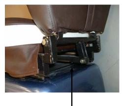
The default angle is good enough. But if new adjustment is needed, then rotate this beam to desire angle of the back.
