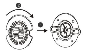
Align jet cover on the jet housing then turn clockwise to install jet cover
