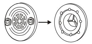
Align and snap the jet inner cover, the suction control screen on the jet cover. Then snap on the jet cover in th arrow direction to the housing to close
