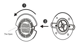
Align fingers to the open, turn counter-clockwise and pull in the arrow direction to remove jet cover
