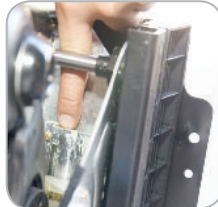
6. Also apply grease at the joints of robotic arms.
