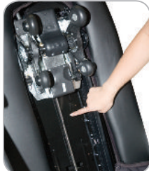
5. Apply grease along coiled pole and at the very bottom of pole. Use remote to move mechanism down, and grease top of pole.
