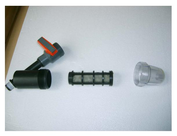
When maintaining your fountain, you will need to remove the mesh filter from the plumbing housing and clean it with warm soapy water and a brush to eliminate sediments. To assemble it, the male end of the mesh filter goes inside the black housing and the end with the rubber ring goes against the clear acrylic cap. You don't need to apply pressure to the cap by screwing it to tight when installing it back.
