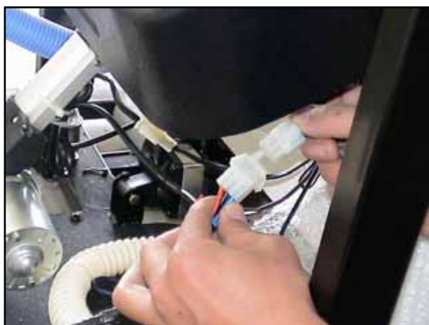
Step 11: Connect the jacks of electric wires.
