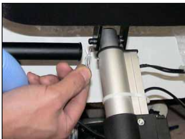
Step 9: Insert an "R" clip in to the #2 pin to fix it.
