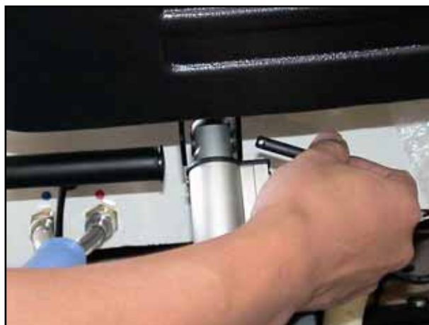
Step 8: Insert #2 pin into the holes on the "U" and the reclining motor to join them together.
