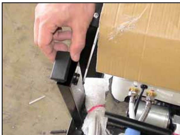
Step 7: Insert pipe plugs into both rectangle pipes.
