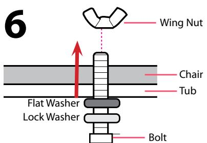
Install bolt and washers in order shown here. Tighten wing nut to end of bolt by reaching underneath the chair. Use a wrench to secure.
