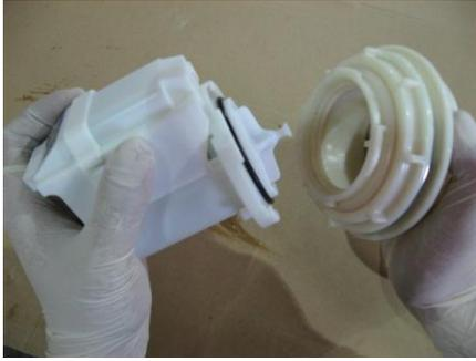
**Step 1:** Disassemble Jet: Pull off “pin lock” Twist motor pump “clockwise” to detach housing and pump. Remove the lock Nut
