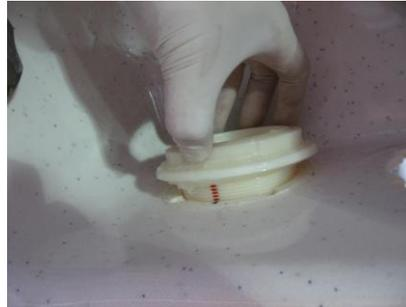
**Step 8:** Install Pump housing: Insert Housing and Adapter onto the pencil circle marking
