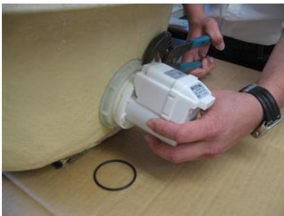
**Step 11** Holding housing: Remove the rubber gasket from motor pump. Lock pump to housing “counter-clockwise”. hold pump tight while tightening the lock nut
