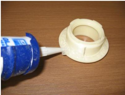
**Step 7:** Apply **second layer** of silicon on top of the ring as picture shown Use finger to smooth silicon as needed
