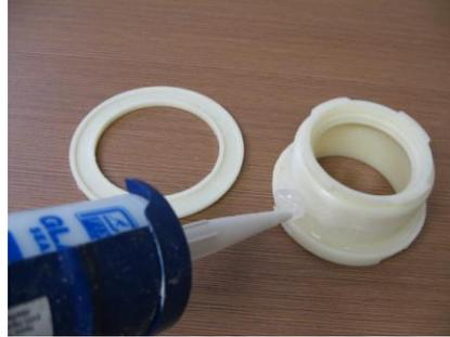
**Step 5** Apply **good amount** of silicon on plastic housing as picture shown above
