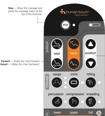
Power – Lights to indicate that master power switch is on.
