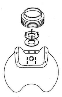
2. Turn over the basin , remove the nut (M17) fitting on the screw of basin and put the tilting mechanism on the basin and then tighten thenut to fix the mechanism to the basin.
