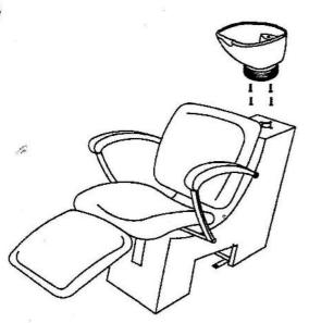
and make sure the serow of mechanism is in the hole if base. Then adjust the angle of basin to expected position. Then fix the basin to the base with nut and two washers which are removed in first step.
