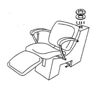
1. Open the back cover of base, unscrew the nut (M14) and two washer (one is round and the other is square) which connect the tilting mechanism and base then remover the tilting mechanism.
