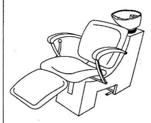
3. Put the basin with mechanism on the base 4. Install the fixtures as in structions and connec the pipe with the drain and make sure no liaking At last fix the back cover of base.
