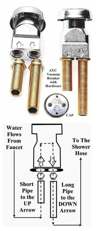
A vacuum breaker is an attachment that prevents water from being siphoned backward into the public drinking water system.
