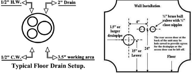
Scenario #1 = typical floor setup for the drain and water lines. Scenario #2 = typical wall setup and dimensions for the drain & water lines.
