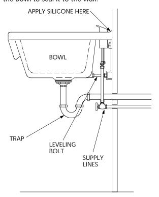
12. Mount the Bowl onto the Wall Bracket by lowering the Lugs on the back of the Bowl into the Wall Bracket.
