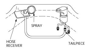
If your Bowl is equipped with a Vacuum Beaker, connect one end of the Fixture Hose to the inlet side of the Vacuum Breaker. Connect the other end to the Fixture Tailpiece. Attach the Spray Hose connector to the Vacuum Breaker outlet.
