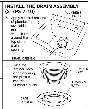
9. From the underside of the Bowl, place the Fiber and Rubber Washers over the Strainer Body. Secure the Strainer **BOWL** Body with the Nut.
