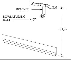
13. Check to be sure the Bowl is level side-to-side and front-to-back. Connect the Fixture to the hot and cold supply lines. Install the trap and connect the drain. Apply a bead of silicone to the back edge of the Bowl to seal it to the wall.
