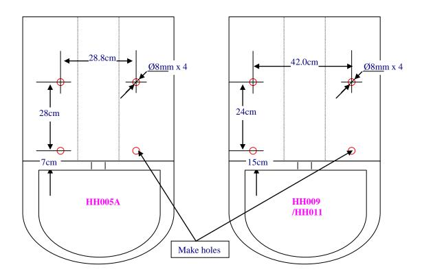
Fig. 1 Installing holes position for Swivel
