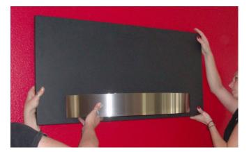
Screw in the two smallest screws to secure the unit to the wall. These screws have one small washer each. Align the vertical mounting tabs at the bottom of the fireplace with the screw holes, thread and tighten the screws to secure.
