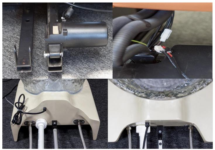
Mount the rear of the drain pipe to the drain mounting bracket using the smaller clevis pin and clip.
