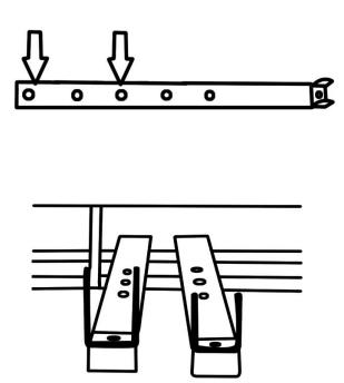
**Installing Basin** - Mount the motor to the bracket using the large clevis pin and clip. Connect the 2 wiring harnesses (1 black and 1 white) to the spa chair, Turn on spa chair and push and hold the left arrow button to send the push rod forward until it stops.
