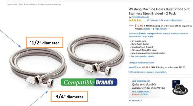
Use <u>Stainless Steel Braided</u> Hoses for Washing Machine with the  $\frac{1}{2}$ " diameter hose and  $\frac{3}{4}$  4" fitting at the end of the hose.
