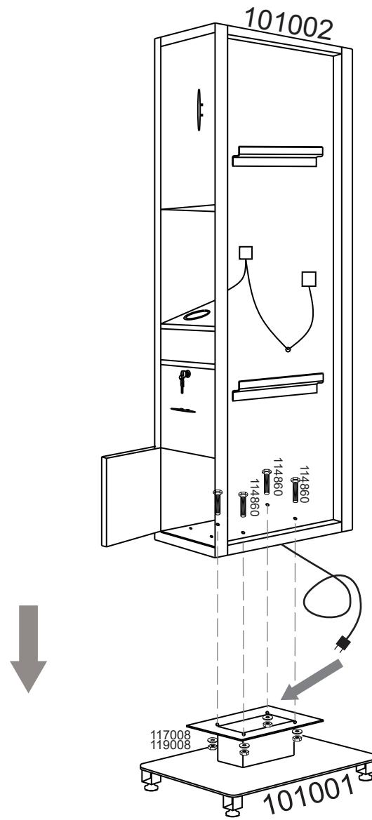
The plug passes through the center of the base.
