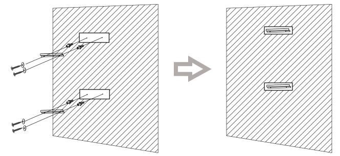
Secure the bracket onto the wall with provided expansion bolts, then secure the mirror onto the metal bracket. DIR's expansion bolts are meant for solid (cement or solid wood) walls, please use appropriate expansion bolts or wall anchors for your mounting needs.
