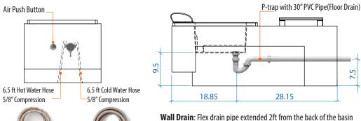
**Wall Drain**: Flex drain pipe extended 2ft from the back of the basin **Floor Drain:** Drain pipe & bushing extended 3" from the back of the basin
