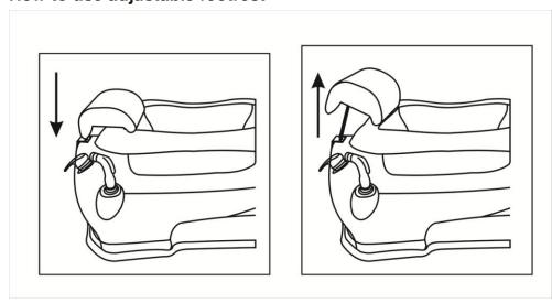
Place left hand on the back of the footrest and gently Pull upt as shown picture1.
